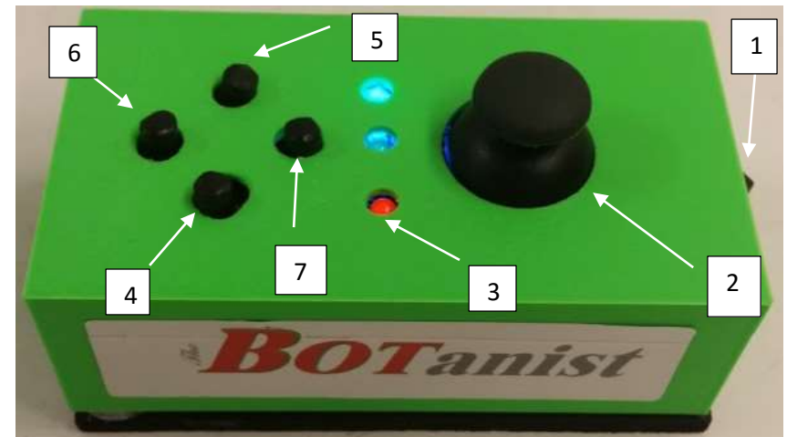
Robot Controller: (1) Power Switch, (2) Joystick Control/Button, (3) Status Lights, (4) Arm Up Button, (5) Arm Down Button, (6) Claw Open Button, (7) Claw Close Button
